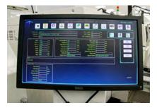
Using Windows operation interface and easy to learn for user, with good man-machine interactive function. Programming is designed with teaching and navigation function; guidance is available on every step. Operating Journal/Breakdown Record/Breakdown Diagnosis.
