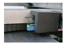
Uniform ring light, high brightness coaxial light and advanced upper/lower vision system. Full range of light compensation, automatic and accurate recognized of all type MARK points. Applicable for tin plating, copper plating, gold plating, tin spraying, FPC and other types PCB with different colors, able to ensure high accuracy.
