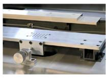
Three axes linkage is designed with super-high dynamic characteristics. It can quickly adjust the PIN jacking height of PCB with different thickness.
