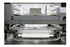
Stencil cleaning system is automatic and effective. Three options of Dry, Wet and Vacuum cleaning can be selected to use, also clean manually. The unit to clean is separated from CCD camera, which can minimize the load of motor and impulse, improve the positioning precision and speed and extend the service life. Sprinkler system ensures spraying evenly from top to bottom.
