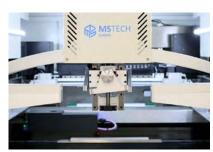
It is applicable for stencils of various sizes. Automatic stencil positioning system saves the line changeover time and enhances the overall efficiency.
